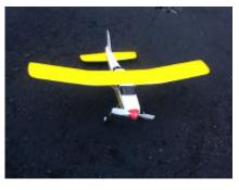
The wingspan is about 10 inchs. It is powered by one small nicad cell which is charged by connecting a 2 cell AA battery pack to it for ~ 2 minutes. John would stand in the middle of the runway and hand launch it and it would circle around his head
