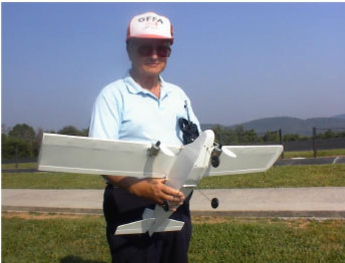
his " All Two Yards ". This one is powered by a couple of 280 electric motors wired in parallel to 10 nicad cells . The model is very fast and highly maneuverable. I can't wait to see what he will come up with next.
