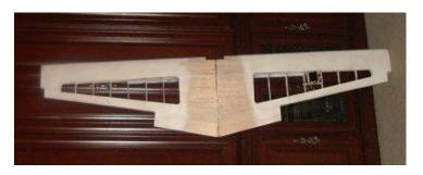
his previous endeavors. The construction has lots of fiberglassing. He is completeing work on the wing at this time. He says that the wing has a span-wise airfoil and has built in wash-out.
