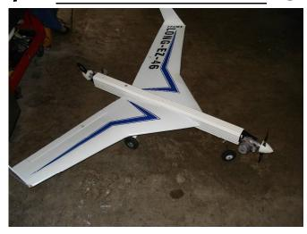
Bud Weisser is at it again! Above is his "DreamPipe". A twin powered piece of plastic downspout. Bud gave specs as follows; Empty wt.:3 lbs., Useful load :1 lb., Gross wt: 4lbs., Rate of climb/2engines: 1000ft/min, Service Ceiling:5000Ft., Vne:(?) estimated 150kts, Mach.17, Stall Speed: estimated 20kts, Engines: two(2) Turbo Compound Magnum .48....
