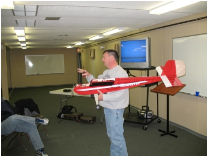
Scott with the camera/downlink equipped, electric powered, Junior Telemaster.
