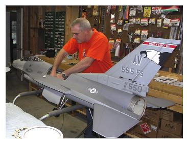
The F-16 is powered by a JetCat P160-SX turbine, which produces 36+ pounds of thrust at 125,000 RPM and features kero-start ignition. All-up weight (dry) should be in the neighborhood of 30 pounds, so the jet should have plenty of power for fast straight-and-level flight and big verticals.
