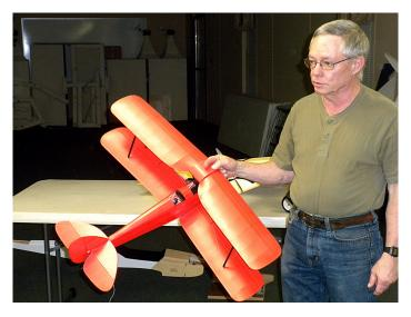
shrinks with heat. The rest of the setup is a 10Amp ESC and 8x3.8prop on an unknown kv motor. This 3 channel plane "flies like a pussy cat" and gives him about 20min of flying with his setup.
