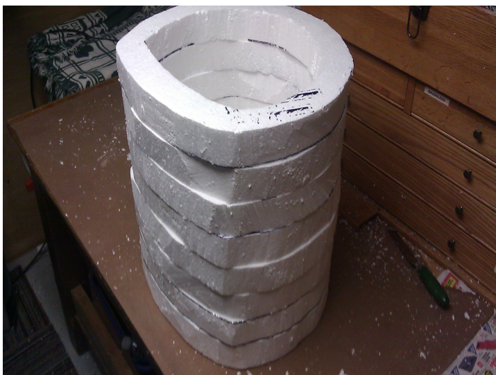
Illustration 1: This shows how Rick is building up the fuse.
