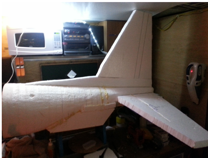
Illustration 2: This shows the roughed-in tail plane.
