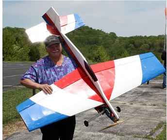
▶ Bill Leonard is keeping me up on field activities. The picture above is of David Johnson and the Mojo 65 he built., It's kitted by Swany's House. Its a big model at 71 inch wingspan and David opted for electric power. He uses two 5000 ma LiPo's and a160 amp speed controller powering the large EP motor driving a 19-8 prop.
