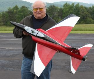
ducted fan. The battery is a 6 cell, 5800 mA. Wingspan is 41".
