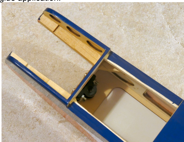
Fig. 3 Nose section of the Falcon 56 fuselage, showing access to both sides of the firewall to check the factory glue job.
