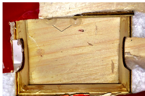
Illustration 1: This shows the wheel mount receptacle in the wing of the ARF Dirty Birdie, with hot-melt glue pooled in the bottom (black lines).
