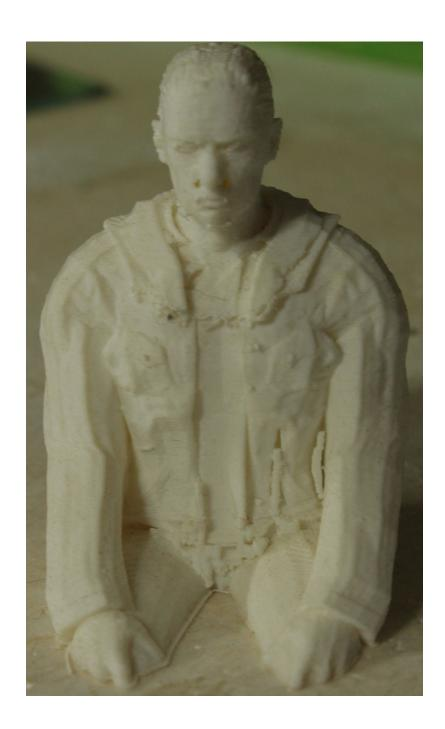
The second figure is printed at 1/10th scale and the MakeHuman figure is 'dressed' in a tee shirt with a denim jacket. I did minimal cleanup on the printed figure but one can easily see the level of detail that can be achieved.
