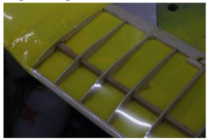
Having a full depth spar provides the most efficient means of getting strength but for this kit the spar was held short of the upper surface by about ¼ inch. Now the strength of a member in bending goes up by the cube of the depth so leaving that 1/4 inch on the table made for a weaker wing. It is such a fundamental engineering principle that it's doubtful that the designer wouldn't have known about it so there must be something else driving the "design decision".
