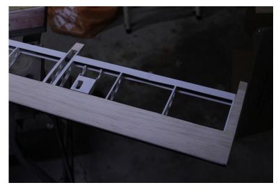
So how does this relate to the spar in the glider wing? I believe it was an attempt by the designer to maximize wing performance by maintaining a smooth airfoil contour all along the wing chord. There is no spar bump to cross. Instead the covering follows the rib contour at the ribs and between the ribs it smoothly changes airfoil contour to a thinner airfoil section midway between the ribs and then smoothly changes back to the rib profile.
