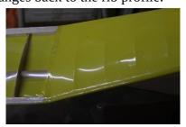
There is probably a design intent to keep the covering from touching the spar and be able to have one piece ribs. If more spar strength was needed the spar could have been made "fatter". While not taking advantage of the cubic relationship, making the spar fatter could have made up for its lack of depth. And also remember it's always nice to make use of standard shapes and sizes to keep costs down.
