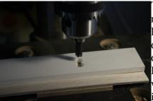
To make ribs, pre-cut rectangular rib blanks, stack them with edges lined up and place them under the drill template. Now use the core drill to drill through the rib blanks. Do not let the blanks shift around when drilling the holes. The result is a set of rib blanks with perfectly
