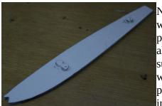
Now is the time to add holes for wing jig rods and/or servo wire passages. I slide my ribs onto 3/8 aluminum rods which are supported as the ends with equal width 2x4's. This makes the rods parallel and if the rib holes are inline then the wing will be
