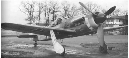
The TA-152 H-1 had a very similar airframe to the FW-190 but in place of the radial engine it had an inverted Junkers 213 EV-12 engine with 35 Liter displacement (2135 cubic inches) with 3 valves per cylinder capable of 3300 RPM. While delivering a modest 1,726 horsepower at take off what made it special was a two stage three speed supercharger with intercooling.
