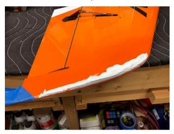
Here's the wingtip after final sanding, and after tiny imperfections are filled in with **Bondo spot putty**. The spot putty is the red that you can see toward the leading edge of the wing.
