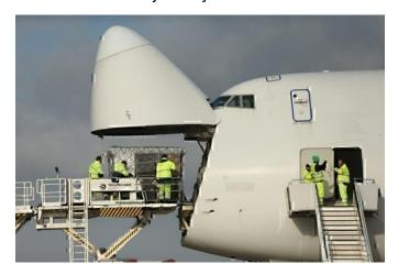
Boeing engineers weren't certain there would be demand for a jumbo passenger jet, so they hedged their bets by designing the 747 so that it could double as a cargo plane. The cargo version has a nose that hinges up and down to accommodate loading. Engineers added the second deck at the front of the plane to get the cockpit above the nose. They extended the hump to include space for a lounge or first-class cabin, and thus was born the iconic shape that we all recognize today.
