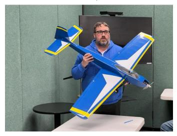
The winning entry came from Warren Oliver, who presented a gorgeous ESM P-40 Warhawk with a 94" wingspan. The model is powered by an RCGF 60cc gasoline engine and is outfitted with electric retracts, including a retractable tail wheel. Test flight coming soon.
