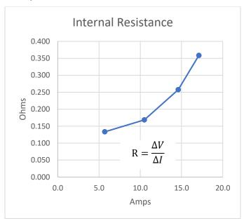
As you can see, the internal resistance went way up and became a strong function of the current. So, this battery went into the scrap bin.
