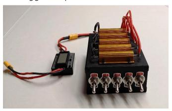
Each resistor increases the current by about 5.5 amps and the battery voltage drops a little. I measured the change in voltage from step to step and divided that by the change in current to determine the battery internal resistance; because the circuit was passive resistors, I didn't have to worry about any other changes. If you decide to make one of these, consider adding a fan and mounting the resistors on a beefier metal plate. I used an old Astro volt/amp meter from the 90's for monitoring.
