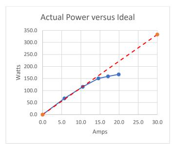
Finally, the internal resistance increased:
