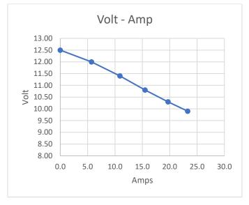
As you can see the voltage drops off as the current increases. You can compare this to a perfect battery in the next graph. The red line is what you would expect from a perfect battery, 3.7 volts per cell, and the blue line is what the battery actually delivered. Not too bad really; the curve starts to drop off at about 160 watts with notable sag at about 225 watts. Not bad for an old brand X battery!
